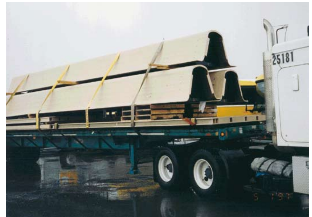
Fig. 7. Molded U-girders (upside down) for INEEL bridge (photo: Martin Marietta Composites).
